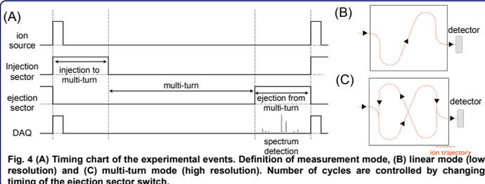
Fig. 4 (A) Timing chart of the experimental events. Definition of measurement mode. (B) linear mode (low resolution) and (C) multi-turn mode (high resolution). Number of cycles are controlled by changing timing of the ejection sector switch.
