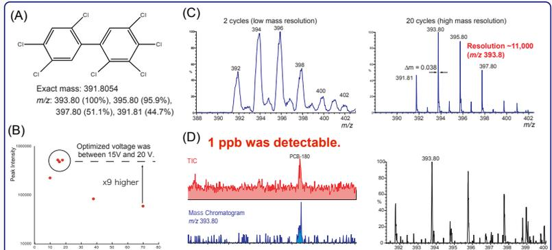
Fig. 6 (A) Structure of C-180S-TP; (B) Optimization of ionization voltage (70 V is typical value); (C) Comparison of mass spectra of PCB-180S-TP (2 cycles and 20 cycles); (D) TIC, mass chromatogram and obtained mass spectrum of m/z 393.8 in 1 ppb.
