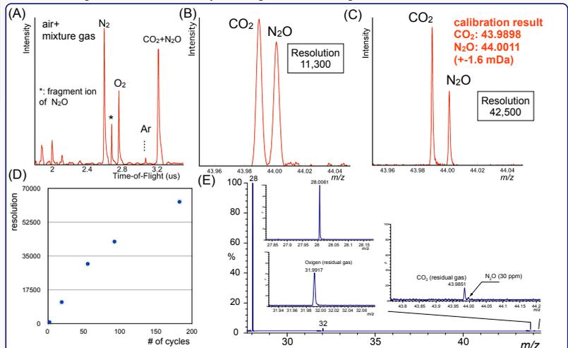
Fig. 5 Separation of CO<sub>2</sub>&N<sub>2</sub>O doublet. (A) control spectrum (air+mixture gas); (B,C) doublet spectra after 20 cycles and 100 cycles; (D) Variation of mass resolution; (E) Simultaneous measurement of N<sub>2</sub> and N<sub>2</sub>O (30 ppm).
