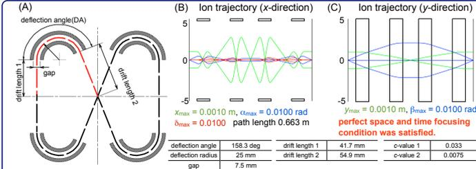
Fig. 2 (A) Ion trajectories in a multi-turn TOF mass spectrometer with the half size of MULTUM II using TRIQ-DRAW. (A) Geometry of multi-turn part. (B) x-direction view, and (C) y-direction view.
