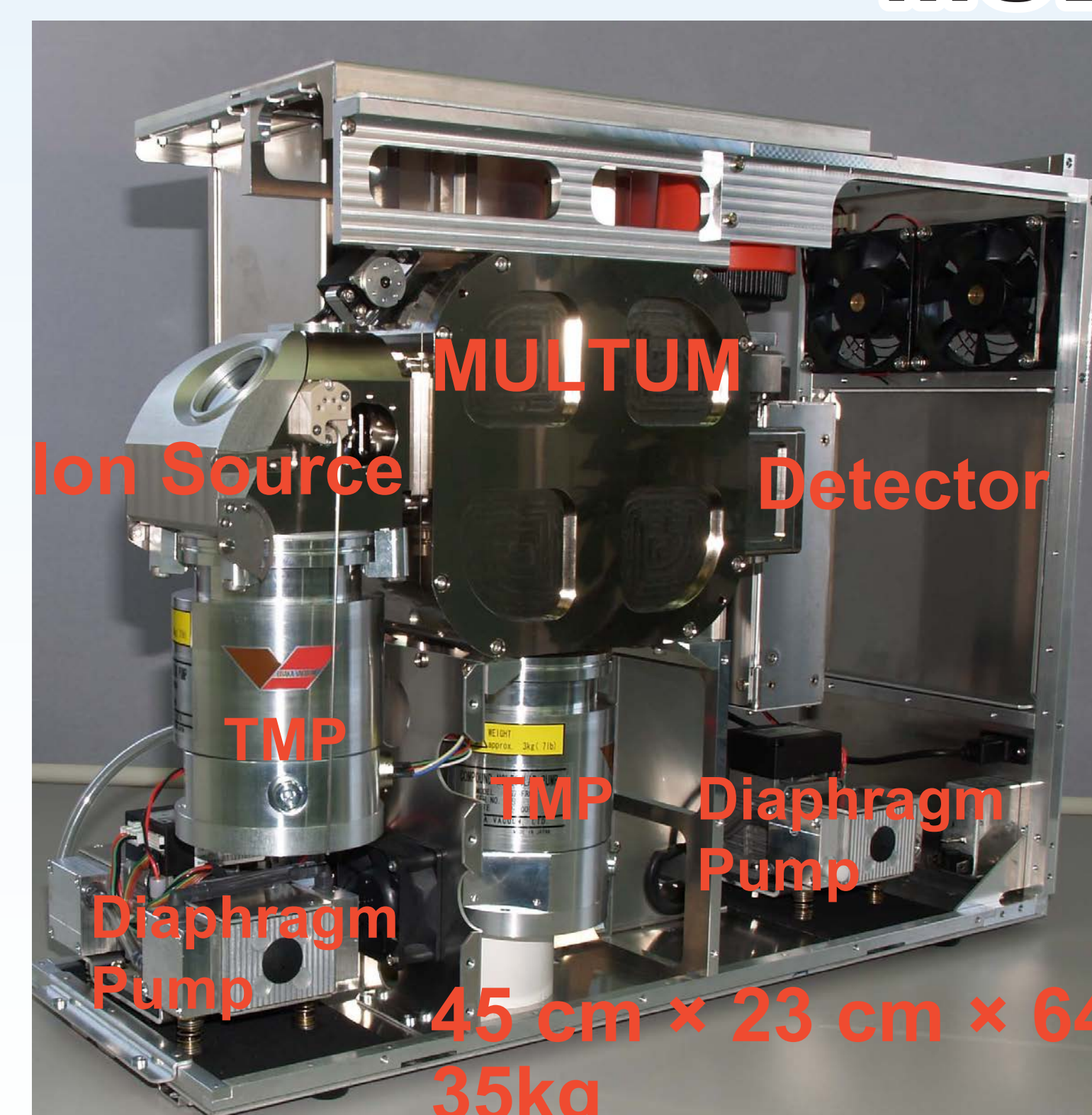
Fig. 1 Photograph of MULTUM-S II. (A) Outside the system and (B) inside the analyzer.
