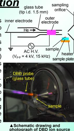
▲ Schematic drawing and photograph of DBD ion source
