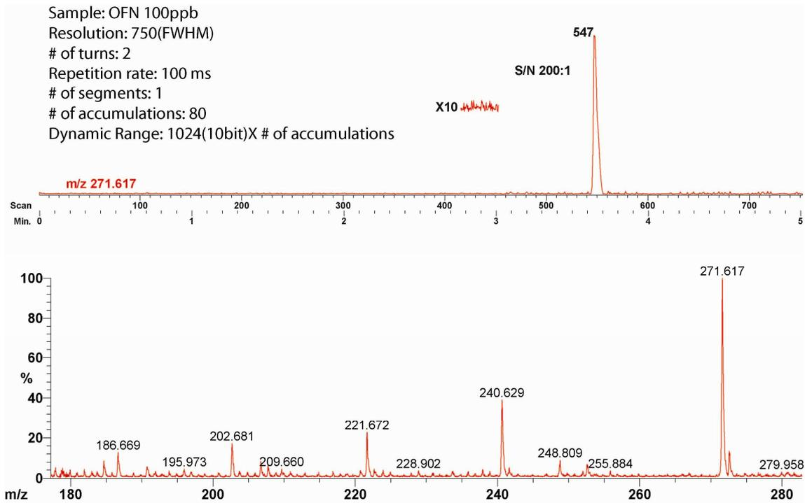
Unit-mass mode is 2.5 turn setting. This is more than enough to get unit resolution up to 500 m/z. Sensitivity is less than linear mode, but it’s still reasonable if you compare to other TOF instruments.
