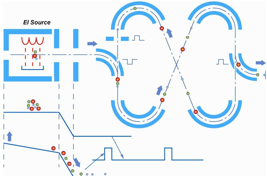
relative to the electrons, “opposites attract”. We won’t say all ions are trapped 100% during standby; however, the duty cycle is no worse than the orthogonal acceleration method.
