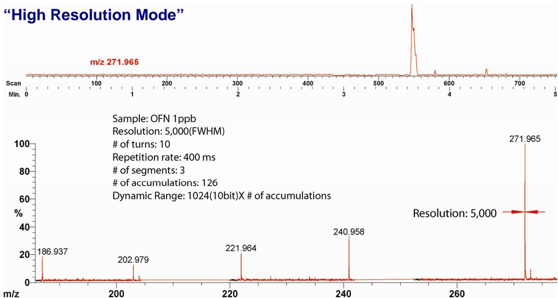
The above mode is high resolution mode. The setting is 10 turns and resolution is around 5000. If you need more resolution, # of turns can be increased.
