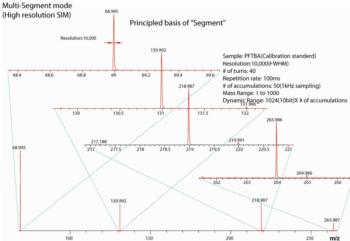
This is actual data acquired in segment mode at 10,000 resolution. Mass range of each segment is narrow but this is a perfect application for monitoring known peaks. In addition file size is kept very small.
