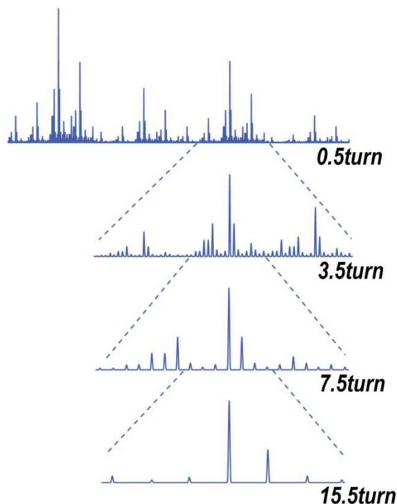
Zooming Mode works well for many applications, but if you wish to have high resolution mode and full mass range simultaneously, “Segments Mode” is the best choice. Our software automatically calculates the range of each segment and then merges them as one spectrum.
